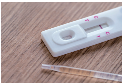
A pregnancy diagnostic device that was able to check pregnancy immediately with a drop of urine was a typical device using early lab-on-a-chip technology.
